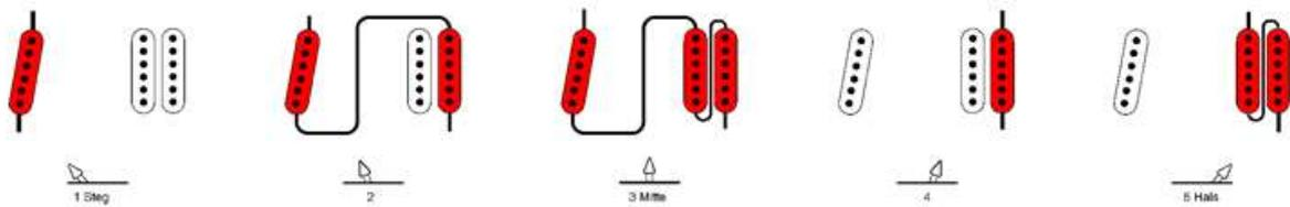
**SH5. Five positions with switching in series, Humbucker splitting, inner coil, Megaswitch M**
