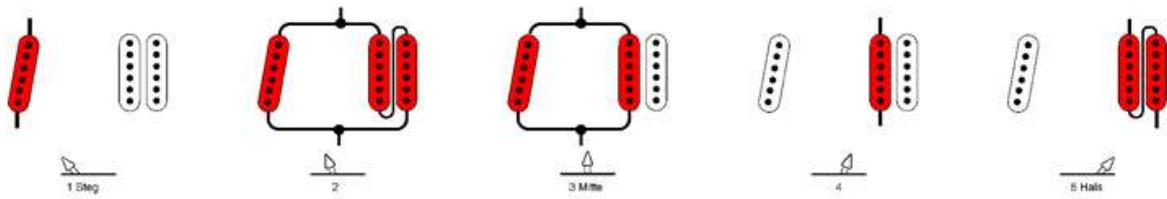
**SH4. Five positions with switching in series, Humbucker splitting, outer coil, Megaswitch M**
